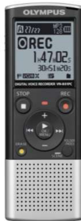
Size: 4.3 x 1.5 x 0.7" 108 x 39 x 16.8 mm Weight: 2.3 oz (66 g), including batteries
